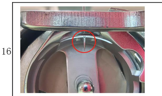
When needle bar in lowest position, the whole needle eye shown in the rotary hook
