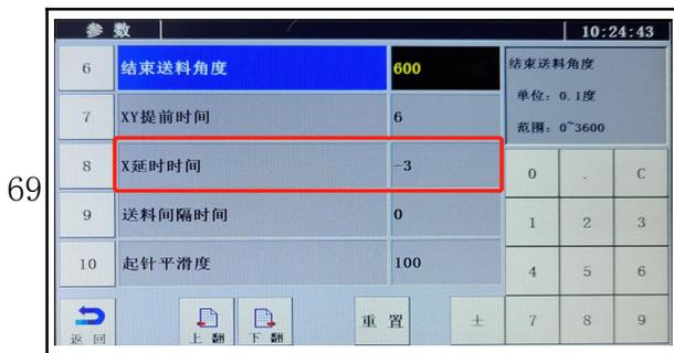
Can adjust 8: X delay time (Normally no need to adjust)
