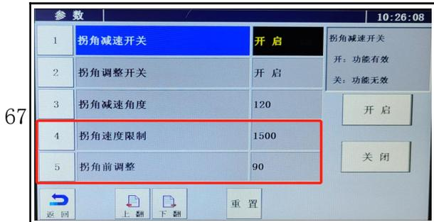
Can adjust column 4,5 (Normally no need to adjust)
