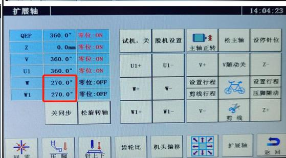
Gap of needle to rotary hook, must check 4 directions. press R- or R+, let the head and rotary hook turn to 90° 180° 270° 360°
