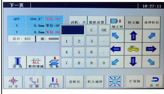
Press the Number area, put the Approximate length of bobbing thread. Unit: mm
