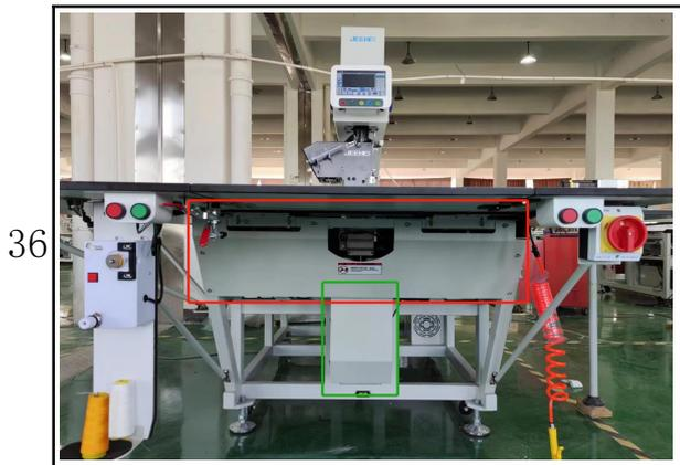
When the gap between needle and rotary hook too big, we can adjust the head (front-back, left-right), to achieve reasonable gap.
