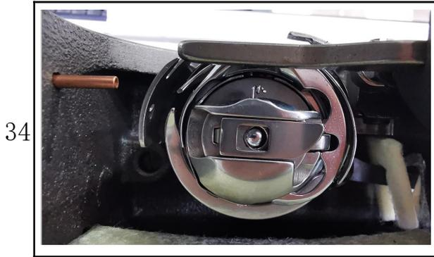
Put the whole bobbin case in the rotary hook
